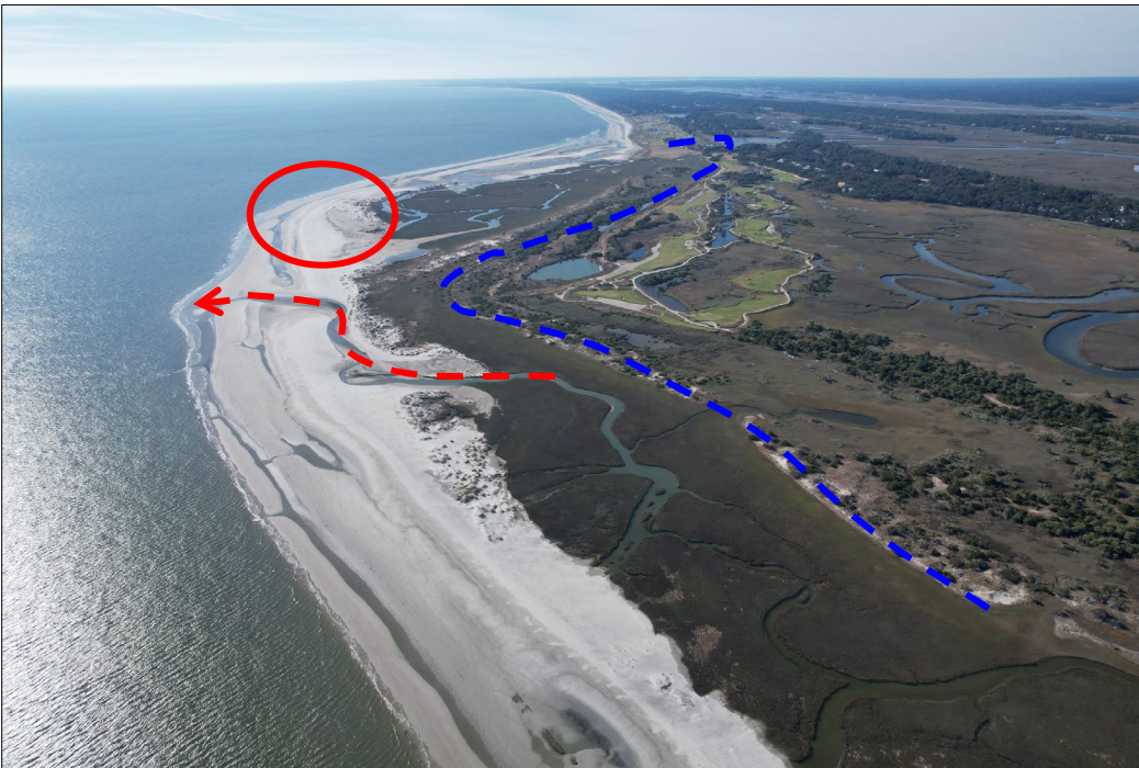
FIGURE 4.8. [UPPER] October 2023 and [LOWER] December 2024 aerial images of the Lagoon Reach. The outer beach is retreating across the salt marsh of the lagoon, occasionally exposing mud outcrops along the wet-sand beach (highlighted in foreground and center of image). The dashed line is the approximate 1989 shoreline. The two flushing channels created by Hurricanes Matthew (2016) and Irma (2017) remained open until October 2023. As of December 2024, the channel on the west end has closed (former position shown with red circle), while the east-end channel has shifted westward but continues to flow in roughly the same locations observed in October 2023 (red line).
