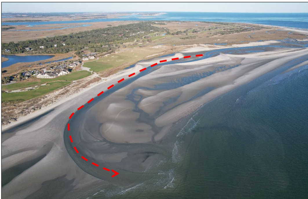
FIGURE 4.7. December 2024 aerial photo over the East End marshes showing the shoal is attaching and feeding sand to the beach between the East End and Stono Inlet (center background). Sand making up the spit on the west side of the shoal will eventually attach to the Lagoon Reach and migrate towards the Ocean Course. A small shallow channel separates the main body of the shoal from the beach as of December 2024, (red line) but it is not expected to inhibit downcoast sand transport over the next several years.
